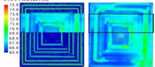
Left: Image of an electric field map of a SansEC sensor. Right: Image of IR thermal data during lightning strike displaying the attachment (where lightning resided on the sensor). This is a rough estimate showing correlation between the high electric field on the sensor to the lightning attachment location.
