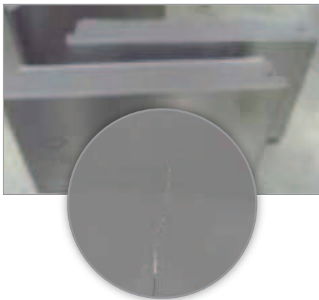
Refrigerator door cover crack failure after temperature cycle
