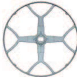
CAD model of optimized four-spoke aluminum-based belt pulley
