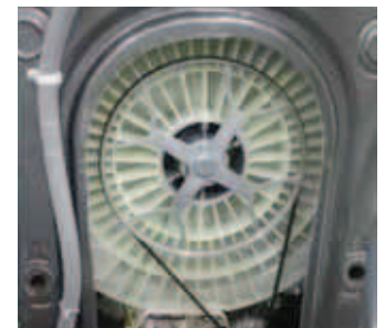
The optimized four-spoke aluminum belt pulley is now in mass production
